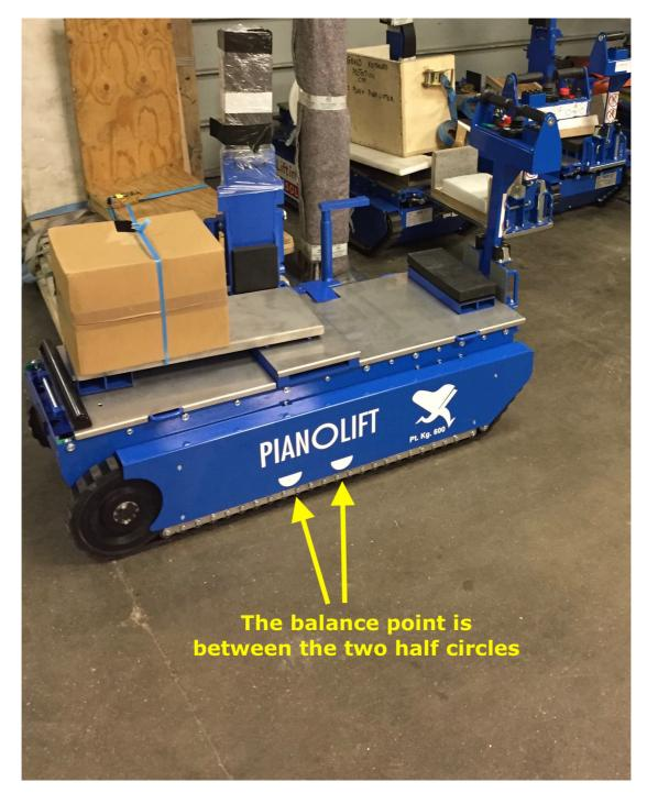
To turn the PianoLift on the center beam the balance of the piano should be between the two half circles, this is also the tipping point when going up stairs.
